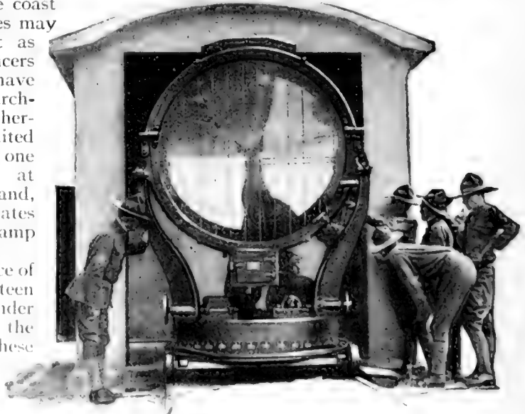
Under favorable conditions the beam from this giant searchlight can "pick up" ships almost six miles distant
